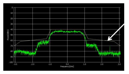
Required spectrum mask at channel 4 of 802.11ad
