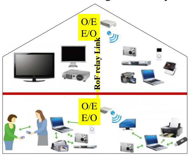
45 GHz and 60 GHz frequencies cannot penetrate walls, floors and ceilings in the buildings.
